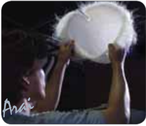
"Bird's nest" shell thickness inspection
